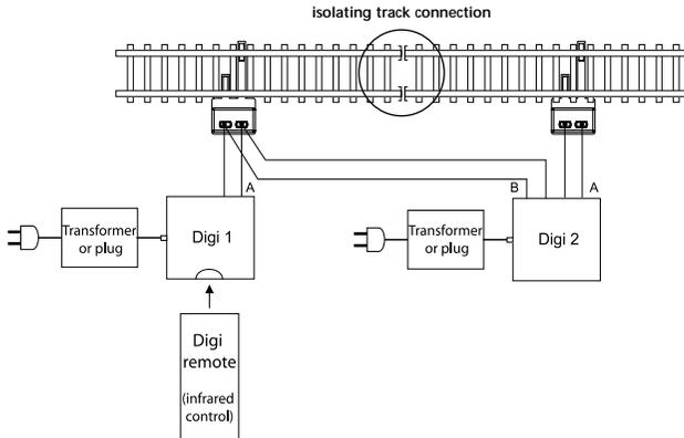
**PIKO Digi 1 extended with two Digi 2 and three isolated rail circuits (maximal level of construction; 10 PIKO Digi 2):**
