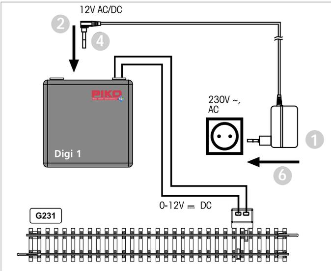
insert the adapter ① into the socket ⑥.
